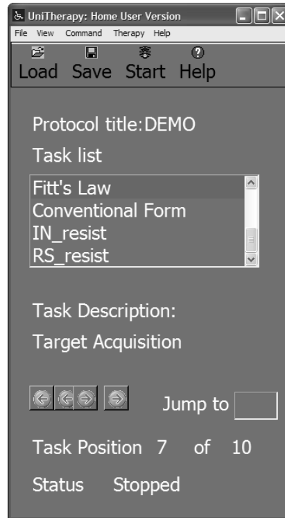
FIG. 5. UniTherapy home user version: designed as a home rehab appliance resembling a CD-player user interface. A user can navigate through the protocol list and select the task; simple voice commands (e.g., “start,” “stop,” “next,” “previous,” “repeat”) are supported, which is implemented using Microsoft Speech SDK; thus the home user can operate via voice command. Certain accessibility features are implemented and are ready to be used for screen-reader application, with more planned, based on usability evaluation.
